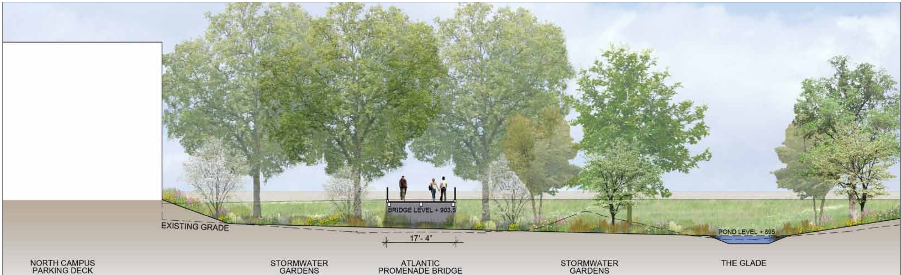
Section through Atlantic Promenade bridge at parking deck. Raingardens collect stormwater and convey it to the Pond
