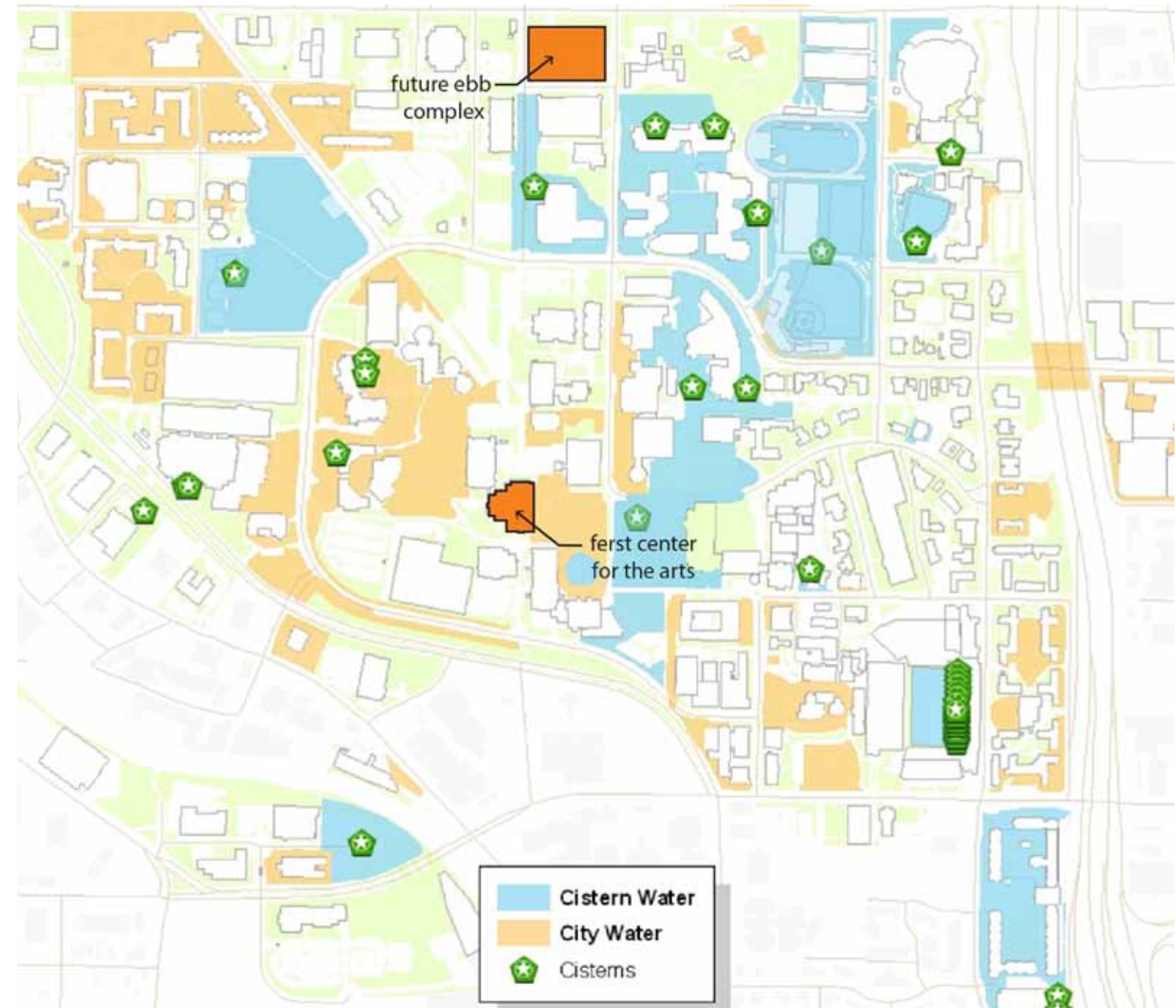
Campus Reuse Water diagram
