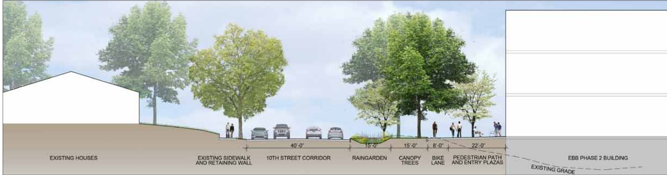
Section A) Proposed typical cross-section through 10th Street with 60' setback
