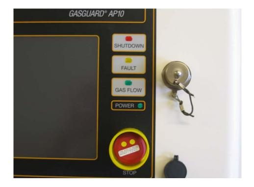
Figure 4.10: AP10 Controller with USB Port Capped
