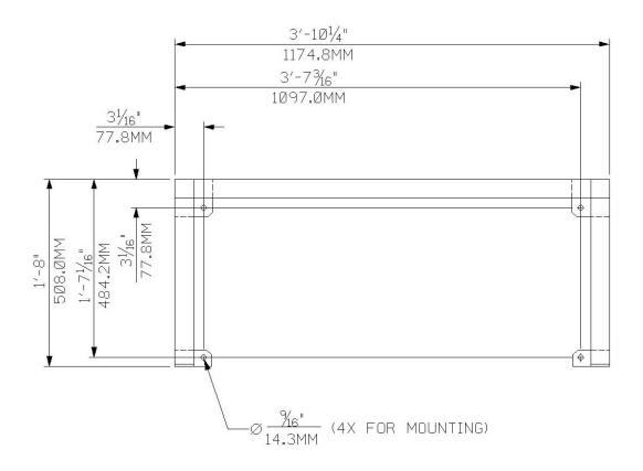
**Figure 2.2.2.5:** Mounting Hole Locations 1x2 Cylinder Rack or 1x2 Cylinder Euro Rack
