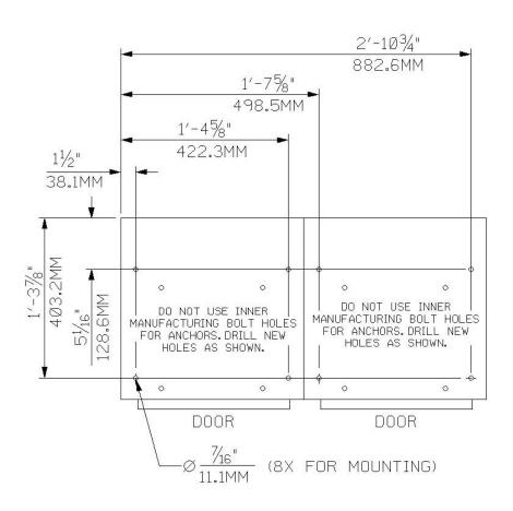
**Figure 2.2.1.4:** Mounting Hole Locations 1x1 Cylinder Cabinet or 1x1 Cylinder Euro Cabinet
