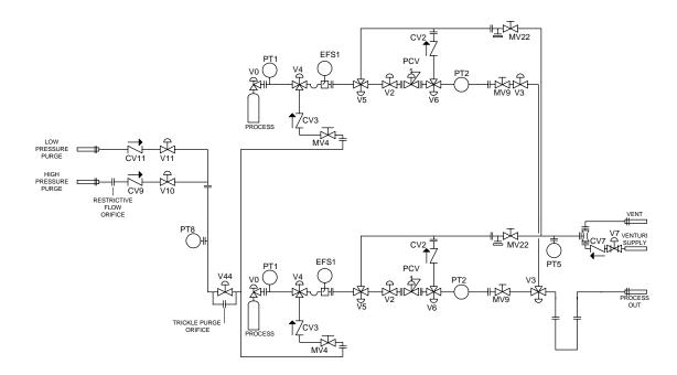
**Figure 7.12:** Example HPLT Piping Schematic
