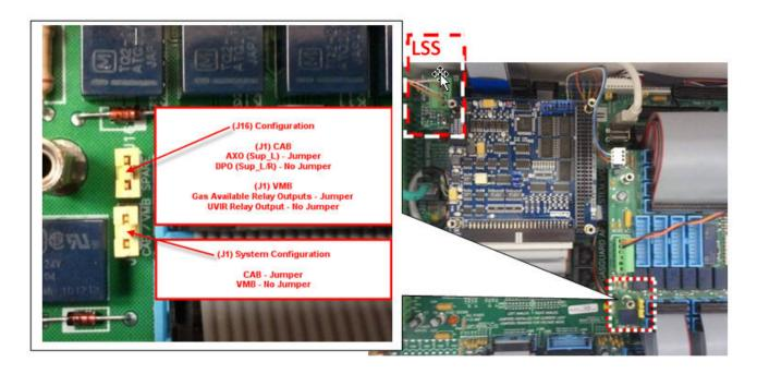
Figure 2 – Jumper Configuration
