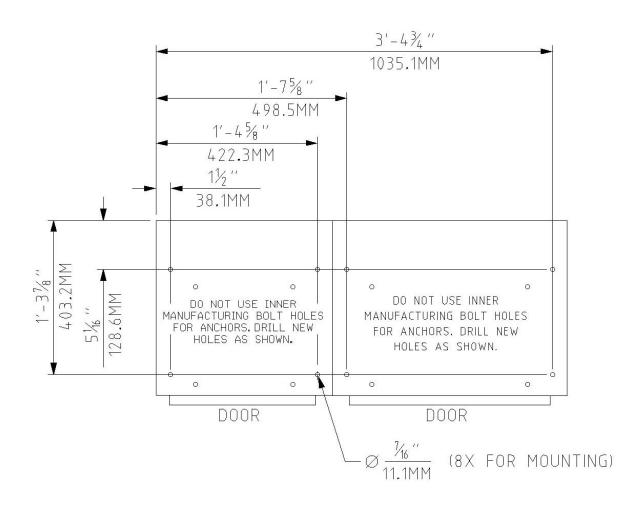
**Figure 2.2.1.5:** Mounting Hole Locations 1x2 Cylinder Cabinet or 1x2 Cylinder Euro Cabinet
