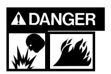
Never attempt to replace a specified gas with another gas without consulting equipment supplier. Incompatible gases could cause fires, explosions or extremely corrosive or toxic compounds.
