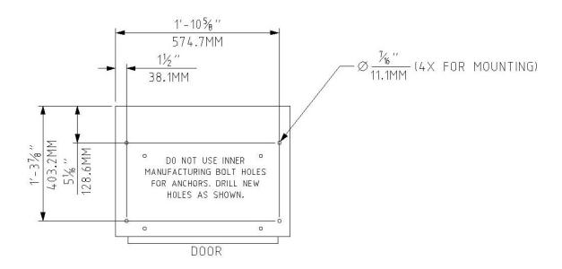
**Figure 2.2.1.2:** Mounting Hole Locations 2 Cylinder Cabinet or 2 Cylinder Euro Cabinet
