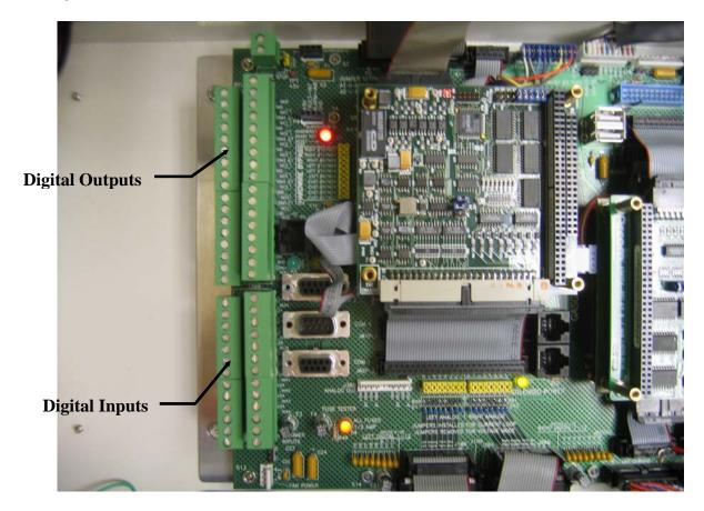
**Figure 4.6:** I/O Terminal Blocks
