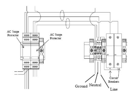
**Figure 4.2c:** Dual Power Supply, Dual Circuit Breaker, Dual Surge Protection Terminal Connection
