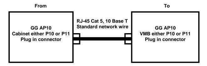
**Figure 4.14:** RS-485 Network Field Wiring Between Cabinets/VMBs
