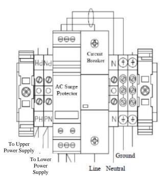
Figure 4.2b: Dual Power Supply Terminal Connection
