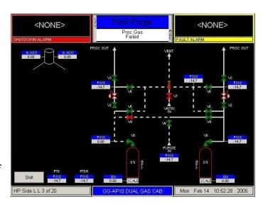
This sequence of evacuation and pressurization will be repeated until the configured number of cycles is completed.
