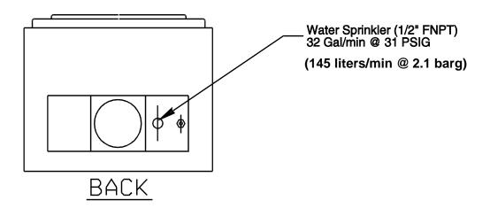
**Figure 3.7:** Sprinkler Connection Location
