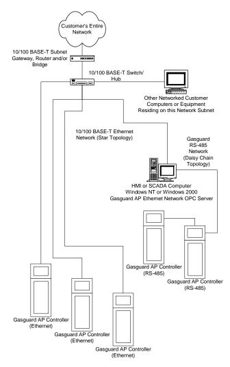
Figure 4.11 Typical GCS Network Architecture
