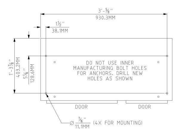
**Figure 2.2.1.3:** Mounting Hole Locations 3 Cylinder Cabinet or 3 Cylinder Euro Cabinet
