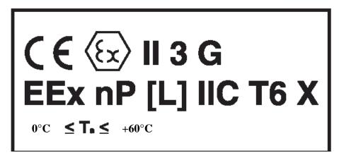
Figure 4.15: AP10 ATEX Label for Systems without a Heater
