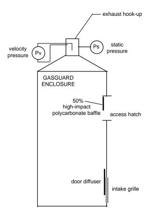
Figure 3.6: Exhaust Hook-up and Ventilation Measurement Location
