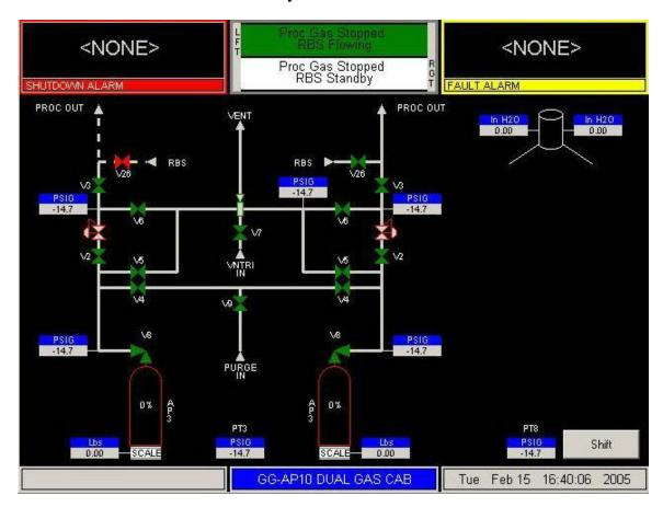
Figure 7.10: RBS Controller Display
