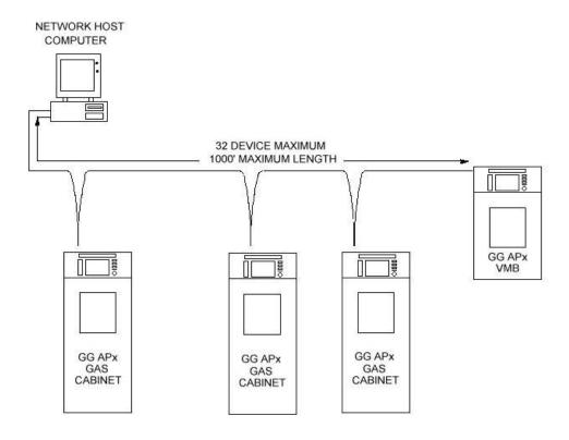
Figure 4.13: Daisy-Chain RS-485 Network Wiring Configuration
