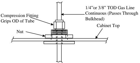
Figure 3.1: Standard Bulkhead
