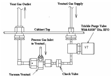
Figure 3.4: Typical Trickle Purge Assembly
