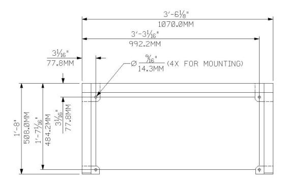
**Figure 2.2.2.3:** Mounting Hole Locations 3 Cylinder Rack or 3 Cylinder Euro Rack
