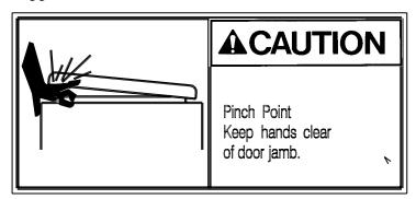
The following label appears on cabinets. It is located on the back of the cabinet, approximately 12" (305 mm) from the top.
