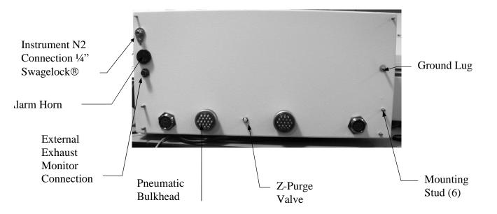
**Figure 3.5:** Rear View of GASGUARD AP10 Controller
