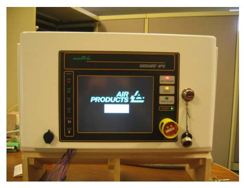
Figure 4.9: AP10 Controller with USB Port on the Face of the Controller
