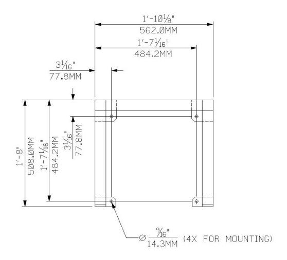
**Figure 2.2.2.1:** Mounting Hole Locations 1 Cylinder Rack or 1 Cylinder Euro Rack
