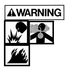
Before attempting to service the system components, close the cylinder valve(s), vent all pressure in the system, and purge all lines that have contained process gas. Tag out and lock out the cylinder valve(s) following the procedure in Safety Section 1.11 of this manual to prevent opening while service is being performed. Once the repairs have been made, follow the start-up procedure, in Section 8.4 of this manual.
