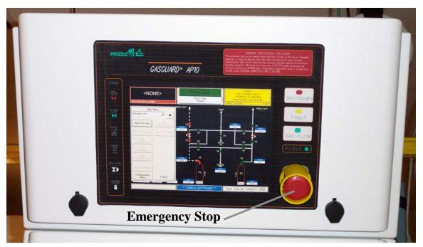
Figure 8.1: Emergency Stop Pushbutton Location
