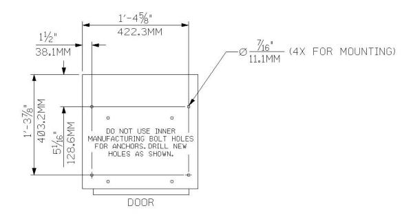
**Figure 2.2.1.1:** Mounting Hole Locations 1 Cylinder Cabinet or 1 Cylinder Euro Cabinet
