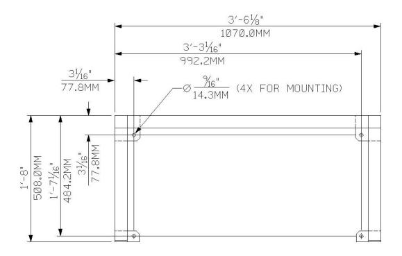
**Figure 2.2.2.4:** Mounting Hole Locations 1x1 Cylinder Rack or 1x1 Cylinder Euro Rack
