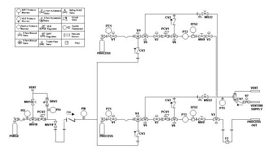
**Figure 7.3:** Process/Process/Purge Auto Crossover Source System Schematic
