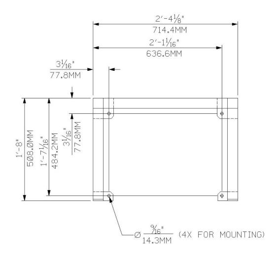
**Figure 2.2.2.:** Mounting Hole Locations 2 Cylinder Rack or 2 Cylinder Euro Rack
