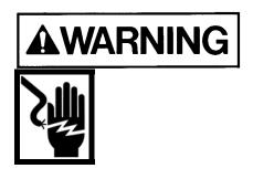
Pressing the "Emergency Stop" button does not disconnect power to the controller. The 120 VAC/240 VAC power is still active within the controller. Do not perform maintenance on the controller without disconnecting or switching of power externally and following the required Lockout or Tagout procedures.
