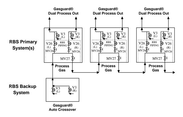
Figure 7.9: RBS - Simplified Piping Interconnections
