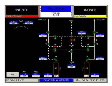
The high pressure tubing will then be "flush" purged.
