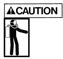
Before approaching a hazardous gas cabinet for a cylinder change, verify that there are no alarm labels displayed on the screen and that the exhaust system is functioning correctly Only operators trained in these procedures and the GASGUARD hazardous gas system are permitted to change cylinders. The appropriate Personal Protective Equipment (PPE) must be worn when performing any Process Cylinder Procedures. See Section 1.9 of this manual for the appropriate PPE.
