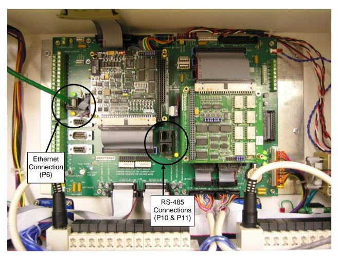
**Figure 4.15:** Bottom View of the GASGUARD AP10 Controller Main Interface Board
