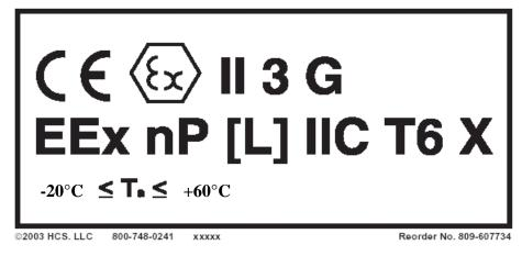
Figure 4.16: AP10 ATEX Label for Systems with a Heater
