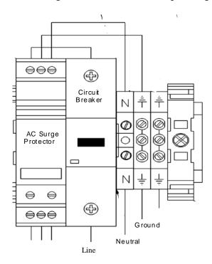
**Figure 4.2a:** Single Power Supply Terminal Connection
